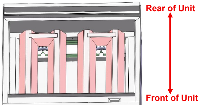
Figure A – Radiants properly installed above burners.
